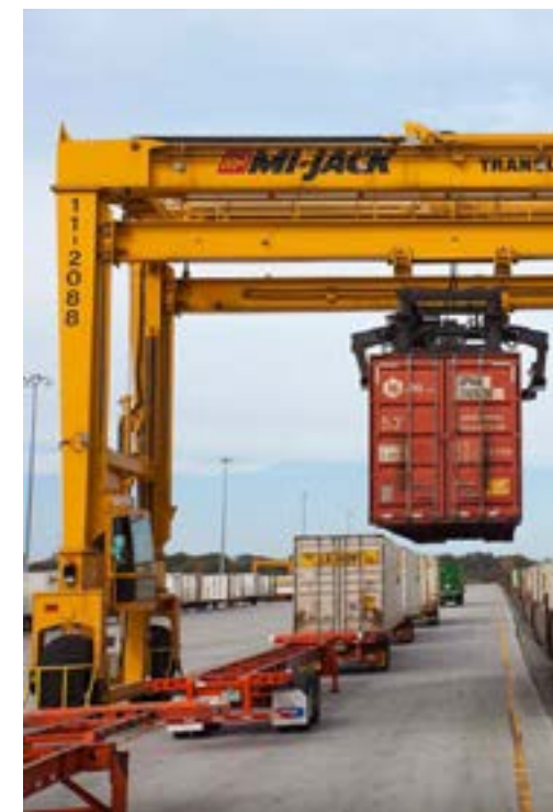
PHOTO: A straddle crane at NS' new regional intermodal facility at Rossville, Tenn., removes a 53-foot domestic freight container from a double-stack train.
